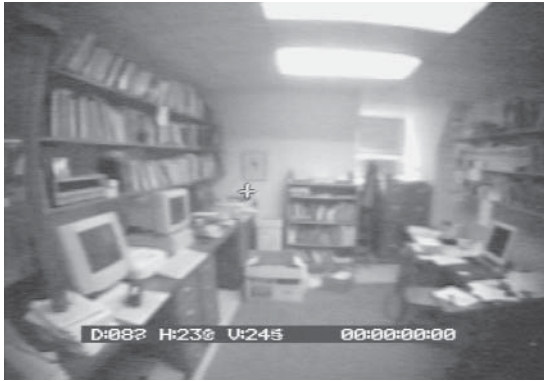
Fig. 1. An example of the scene video as it is output from the HMET hardware with a calibrated fixation cross indicating POR
